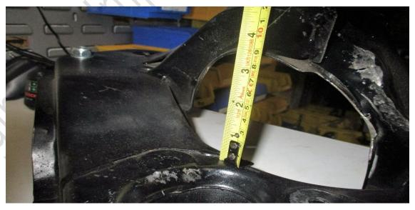
SPACERS CAN BE USED BETWEEN THE SUBFRAME AND THE BODY / CHASSIS RAILS TO GAIN ENGINE INLET SYSTEM TO BONNET CLEARANCE. 1 inch MAX THICKNESS IS ADVISED.
