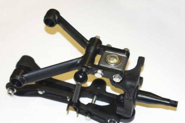
This new balljointed suspension has been developed to offer driving improvements, but without looking dramatically different on the car.
